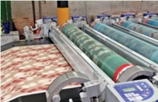
Principe de l'impression rotative / Principal of rotary screen printing
